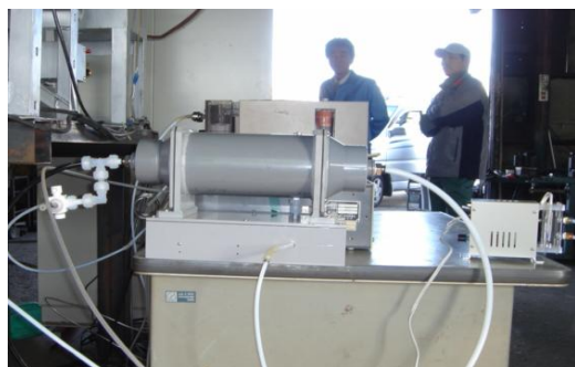
MR-10 A field test for bad smell removal
