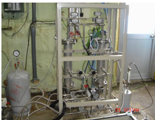
VPSA-CH 4 recovery and purification unit
